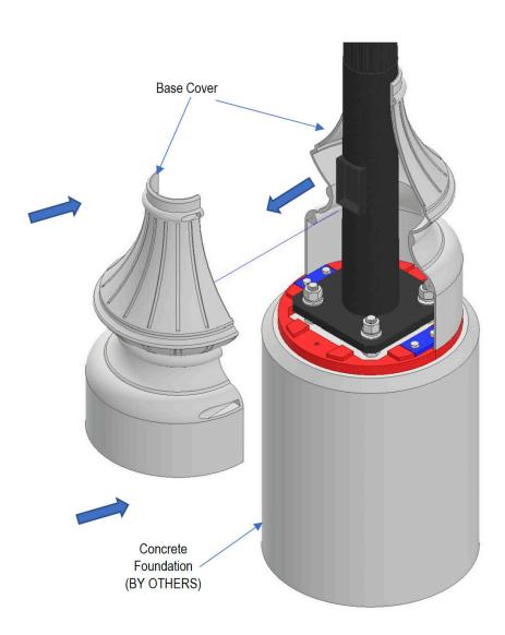
3. Once the Base Cover is installed, Secure by tightening the (4) screws as shown below.
